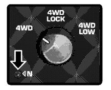
**NOTE:** The 4x4 system will not allow shifts between 4WD/ 4WD LOCK if the rear wheels are spinning (no traction). In this situation a position indicator light will flash and the original position indicator light will remain ON. At this time, reduce speed and stop spinning the
